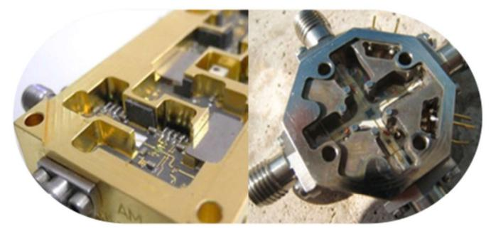
Build-to-spec customized solutions can be provided starting from Customer specifications, including electrical, thermal, mechanical and layout design of single or multifunction microwave components or modules.
